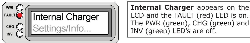
Figure 5-34, Internal Charger Fault
