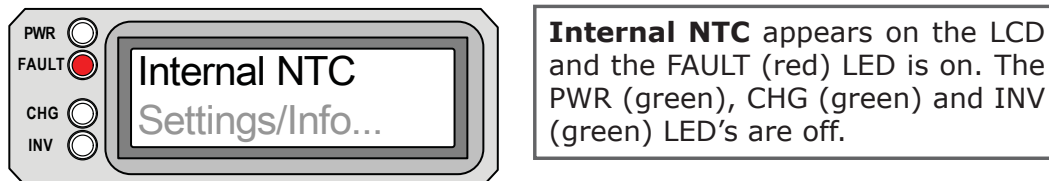
Figure 5-35, Internal NTC Fault
